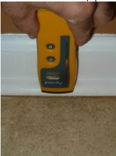
Elevated moisture level, high moisture level, incl. middle part of N wall
