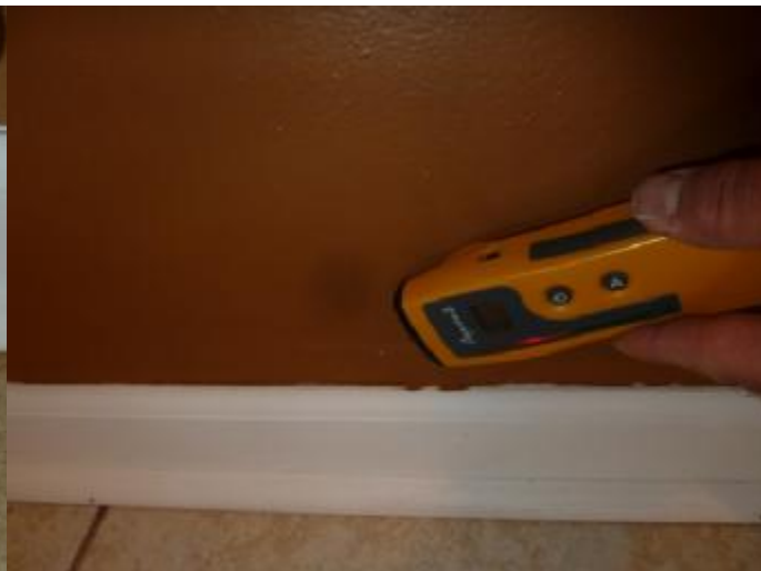
Elevated moisture level, high moisture level, incl. middle part of N wall
